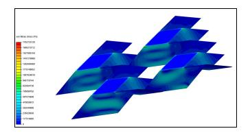
Figure 3 | Zigzag Base Core Stress Diagram. The four top faces endured minimal stresses for compression and shear tests, which prompts inquiry into a kirigami-based variation of the pattern that eliminates these faces. Similar recommendations are made for the square twist core.
