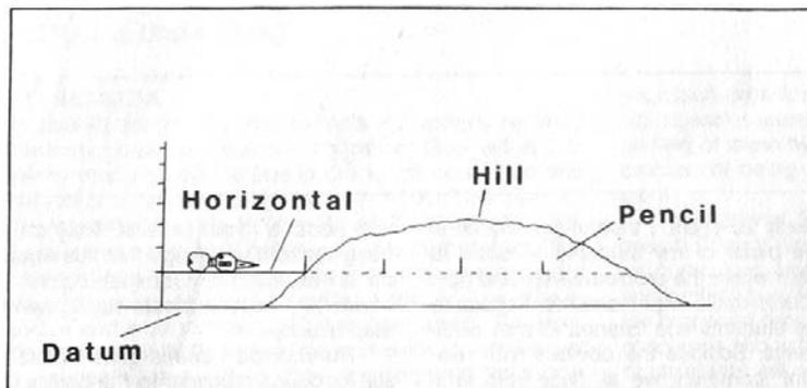
Figure 1. The surveyed hill showing the datum and pencil positions.
