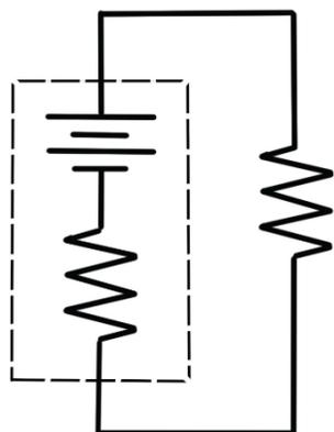
A group of students are to experimentally determine the internal resistance  $r$  of a battery using the circuit created as shown. The battery is assumed to have an internal resistance  $r$  and constant emf  $\mathcal{E}$ . The students are expected to find the internal resistance by plotting their data in a graph. The students have access to equipment including, but not limited to, a variety of resistors, multimeters, and other equipment commonly found in a high school physics laboratory.
