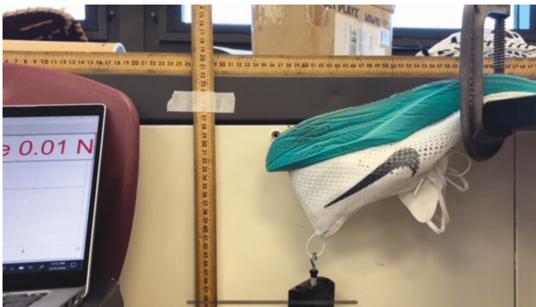
Figure 1. Image of Stiffness Test Setup
