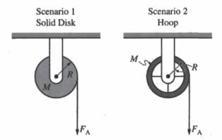
Scenarios 1 and 2 show two different pulleys. In Scenario 1, the pulley is the same solid disk referenced in part (a). In Scenario 2, the pulley is a hoop that has the same mass M and radius R as the disk. Each pulley has a lightweight string wrapped around it several turns and is mounted on a horizontal axle, as shown. Each pulley is free to rotate about its center with negligible friction.
