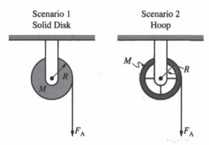
Scenarios 1 and 2 show two different pulleys. In Scenario 1, the pulley is the same solid disk referenced in part (a). In Scenario 2, the pulley is a hoop that has the same mass M and radius R as the disk. Each pulley has a lightweight string wrapped around it several turns and is mounted on a horizontal axle, as shown. Each pulley is free to rotate about its center with negligible friction.
