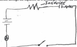
The capacitor is fully charged by the battery. At time t = 0, the capacitor starts discharging through the resistor.
