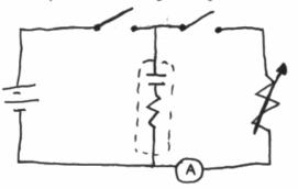
The capacitor is fully charged by the battery. At time t = 0, the capacitor starts discharging through the resistor. Show that the current I through the capacitor as a function of time t is  $I(t) = I_0 e^{\frac{-t}{(R+r_C)C}}$  as the capacitor [=].(e<sup>-\$/Rc</sup>) discharges. R= R++= (R+F2) GO ON TO THE NEXT PAGE. Unauthorized copying or reuse of this page is illegal. Page 6 Use a pencil or a pen with black or dark blue ink. Do NOT write your name. Do NOT write outside the box. Q5133/6
