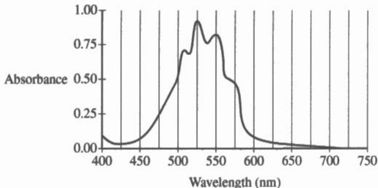
(a) To determine the optimum wavelength for an experiment that measures the concentration of  $\text{MnO}_4^- (aq)$ , the student takes a sample of the solution and measures the amount of light absorbed by the sample over a range of wavelengths. The data are plotted in the graph shown. Identify the optimum wavelength that the student should use for the experimental procedure.
