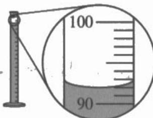
(i) The student uses a 100.0 mL graduated cylinder to measure a certain volume of  $\text{KMnO}_4 (aq)$  stock solution, as shown in the diagram given. What volume should the student record?
