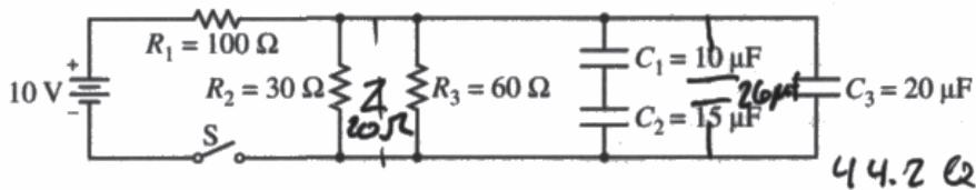
1. The circuit shown above is composed of an ideal 10 V battery, three resistors and three capacitors with the values shown, and an open switch S. The capacitors are initially uncharged. Switch S is now closed.
