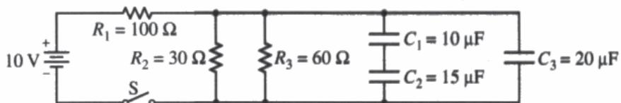
1. The circuit shown above is composed of an ideal 10 V battery, three resistors and three capacitors with the values shown, and an open switch S. The capacitors are initially uncharged. Switch S is now closed.
