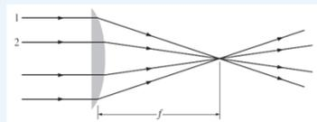
**Quantitative/Qualitative Translation:** The figure at left represents a glass lens that has one flat surface and one curved surface. After incoming parallel rays pass through the lens, the rays pass through a focal point.
