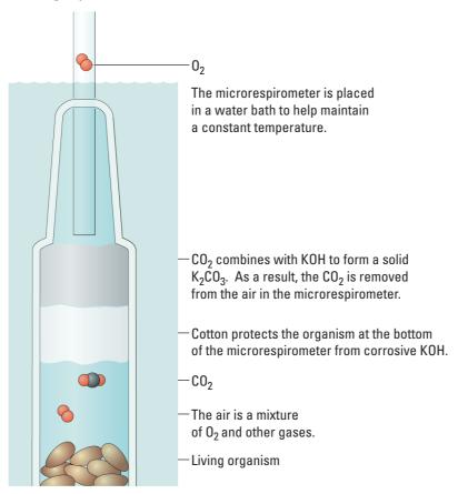
Figure 1. Microrespirometer
