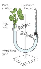
**Figure 2. Potometer Assembly**
