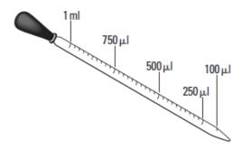
Figure 2. Measuring Volume with a Pipette
