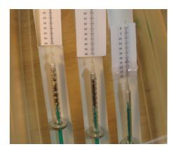
Figure 2. Microrespirometer Assembly
