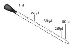
Figure 2. Measuring Volume with a Pipette
