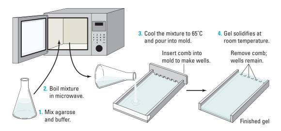
Figure 1. Preparing and Casting an Agarose Gel
