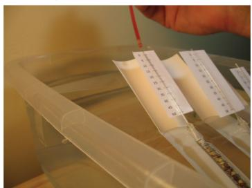
Figure 5. Manometer Fluid Added to Capillary Tube Tip
