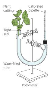
Figure 2. Potometer Assembly
