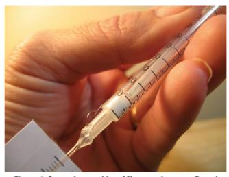
Figure 4. Cotton Inserted into Microrespirometer Barrel
