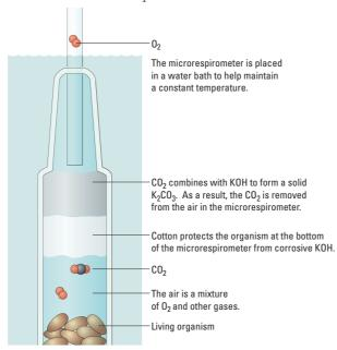
Figure 6. Microrespirometer
