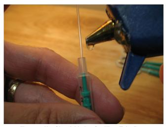
Figure 3. Hot Glue Added to Capillary Tube Base
