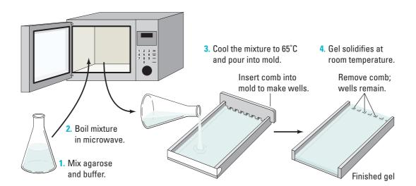
Figure 3. Casting an Agarose Gel
